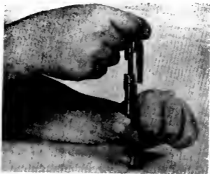
FIGURE 47. REMOVING COCKING PIECE.
